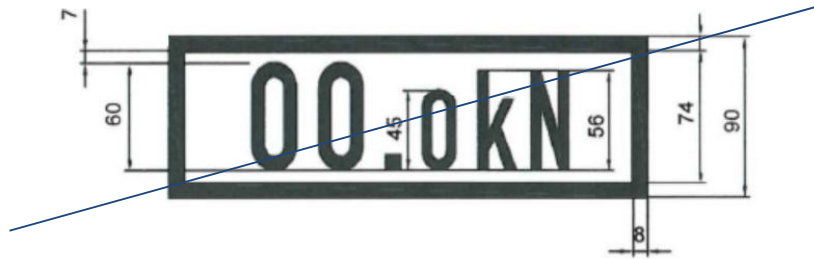
Fig. 4: Marking indicating the braked weight and the holding force in kN on vehicles fitted with screw brakes
