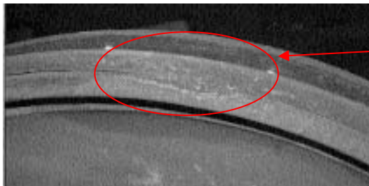
Major irregular crushing of the edge of the wheel rim
